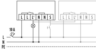
Standard with optional control via a closing button and parallel wiring of max. 8 devices.
