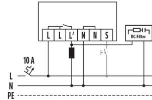
When connecting inductors (e.g. relays, contactors, ballasts) the use of a filter (RC-Filter) may be necessary.
